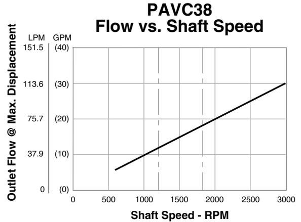
NOTE: Minimum attainable HP setting means that input horsepower will not exceed the indicated setting at the indicated RPM and that the pump will achieve full compensator pressure selected. If setting input power limiter below full flow boundary, full flow may not be obtained at low operating pressure.
