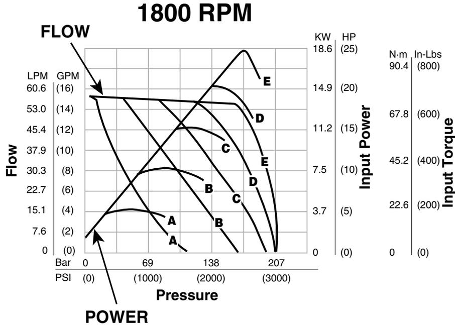
1. Power “A” curve corresponds to flow “A” curve. This represents a particular setting of the power (torque) control.
