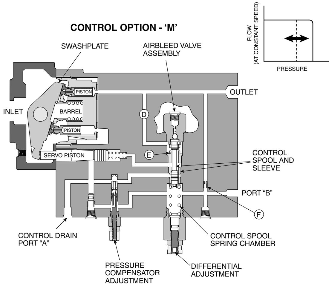
**Pressure & Flow Control (Load Sensing)**
