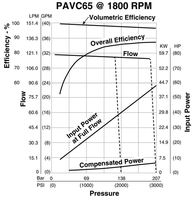
NOTE: The efficiencies and data in the graph are good only for pumps running at 1800 RPM and stroked to maximum. To calculate approximate input power for the other conditions, use the following formula:
