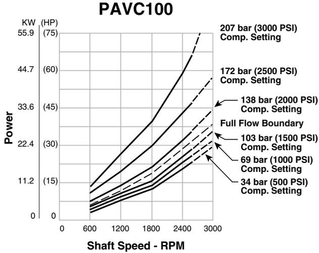
NOTE: Minimum attainable HP setting means that input power will not exceed the indicated setting at the indicated RPM and that the pump will achieve full compensator pressure selected. If setting input power limiter below full flow boundary, full flow may not be obtained at low operating pressure. Determine maximum input power limitation at desired RPM. All points above desired compensator setting curve can be achieved.
