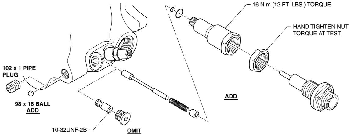
**NOTE:** Install ball through torque port, seat in place through bolt hole.
